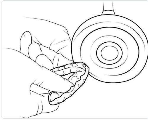
Pre-polish with pumice on dental lathe (muslin wheel, damp)
